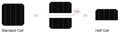
The ribbon length of half-cell is shorter than normal cell. Calculated by Joule's law and Ohm' law, the power loss reduction is nearly 6%.
